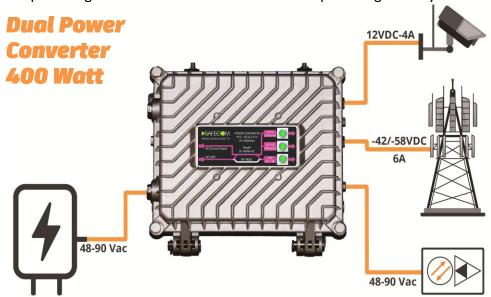
Safecom's new vision focuses on utilizing existing HFC (Hybrid Fiber-Coaxial) networks to power 5G macro and small cells by leveraging the available spare load in the network. This is accomplished through an innovative and highly efficient Dual High-Power AC-DC inverter (400W). The inverter converts AC electricity from the HFC network (typically ranging from 48-90 Vac) into -42/-58V DC, which is used to power 4G and 5G LTE cells.
